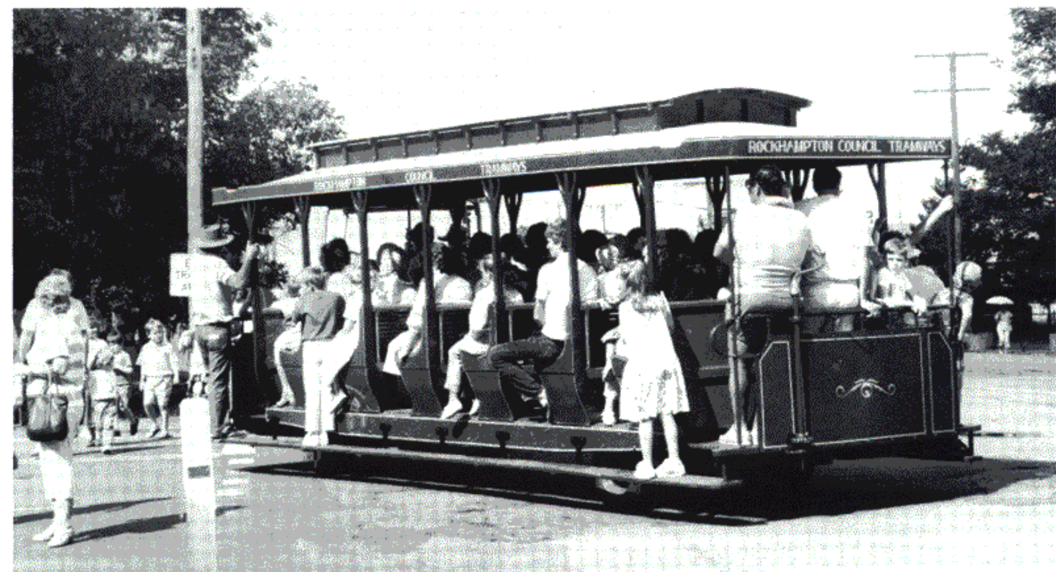
The cross bench horse car at the corner of William and Denison Streets. This tram normally operates on flanged wheels but can be fitted with pneumatic tyres for off-rail running and it ran in this mode during the day hauled by a tractor. KEN McCARTHY
