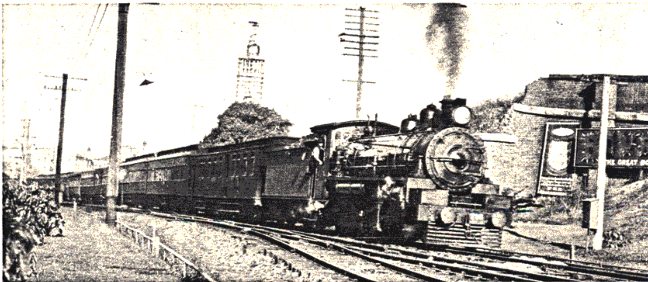
The Western Mail approaching Brisbane's Roma Street station in the early 1930's and headed by C.19-class 4-8-0 No. 798. (Photo: Queensland Railways)
