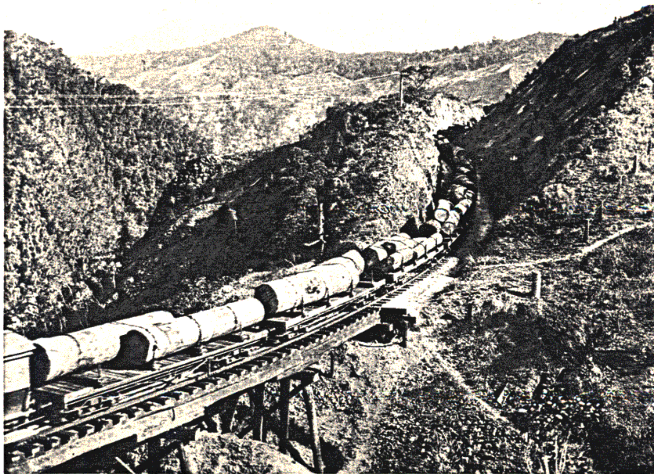
The most spectacular range railway in Queensland is the Cairns Range line. This view shows a B.15-class 4-6-0 negotiating sharp curves on the Barron Gorge section with a descending log train.
