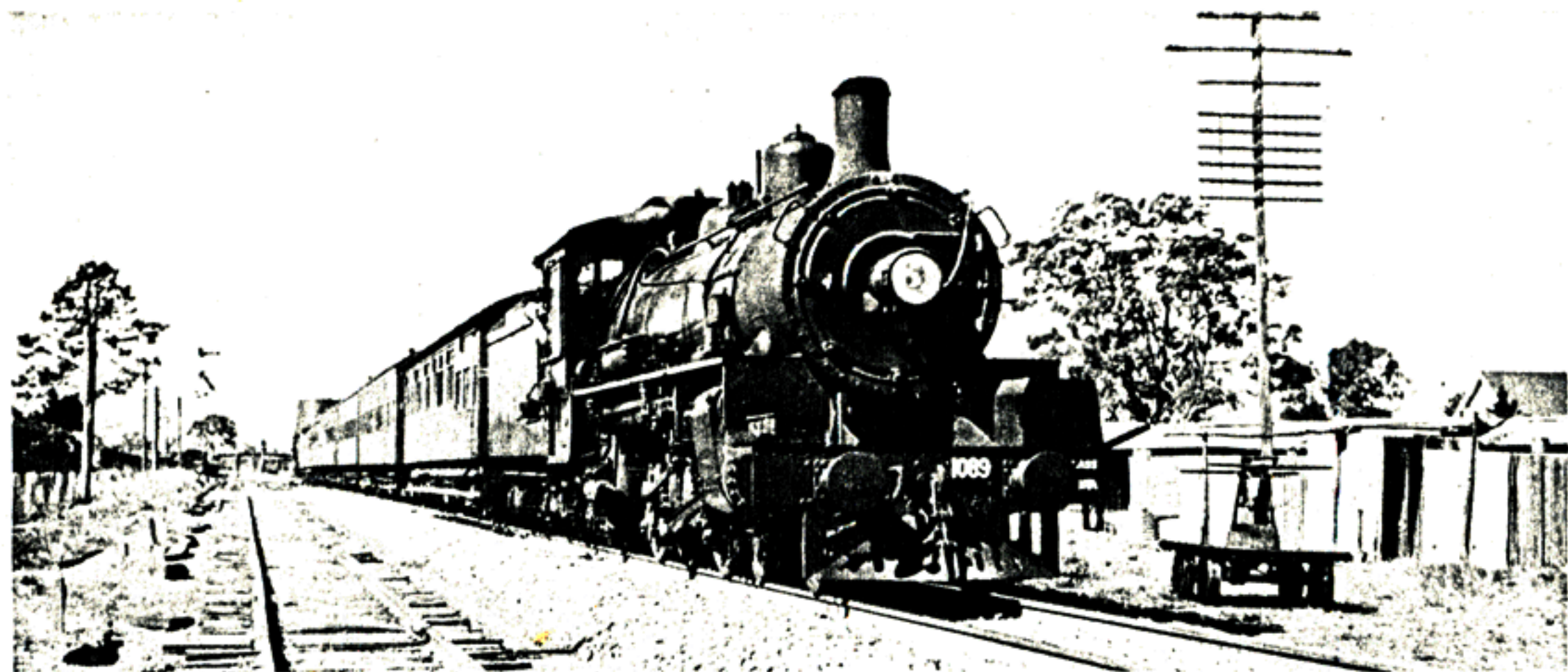
The Queensland Railways' BB.18 \frac{1}{4} -class 4-6-2 No. 1089 leaving Caboolture with an eight-car train for Gympie. (Photo: J. Armstrong)
