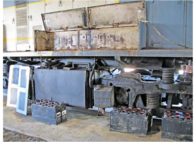
During restoration in Rockhampton: bogies, batteries and battery boxes [ lz 6204]
